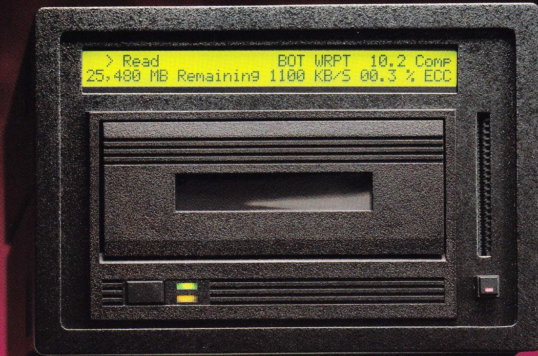
The CY-8500 can store up to 25 GB on a single tape, at speeds of up to 90 MB per minute, completely unattended.
